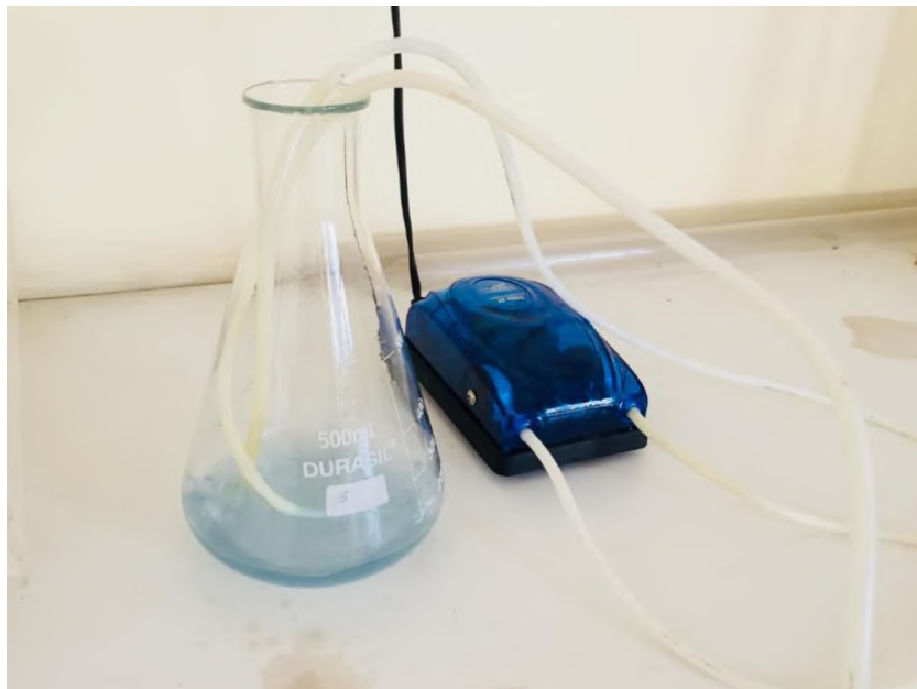
Figure 1: Lab-scale Batch Stripping System
