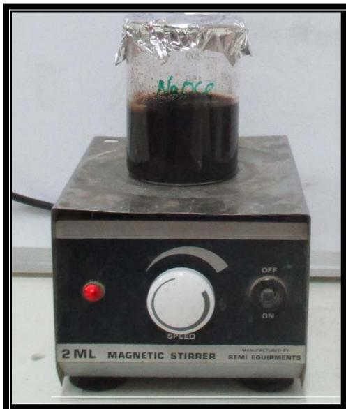
**Figure1: Sample of dye intermediates wastewater in which Sodium Hypochlorite is added.**
