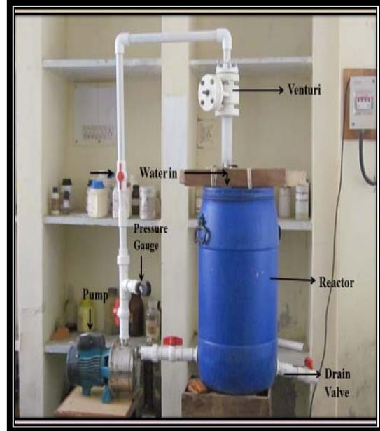
**Figure 3: Hydrodynamic Cavitation Reactor**
