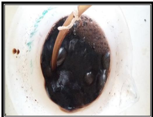
**Figure: 5 Supply of Ozone into wastewater**
