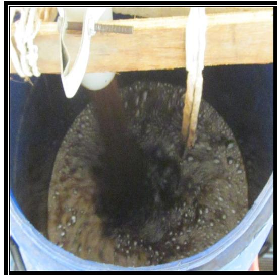
**Figure 4: Wastewater resulting from Venturi back into the reactor.**
