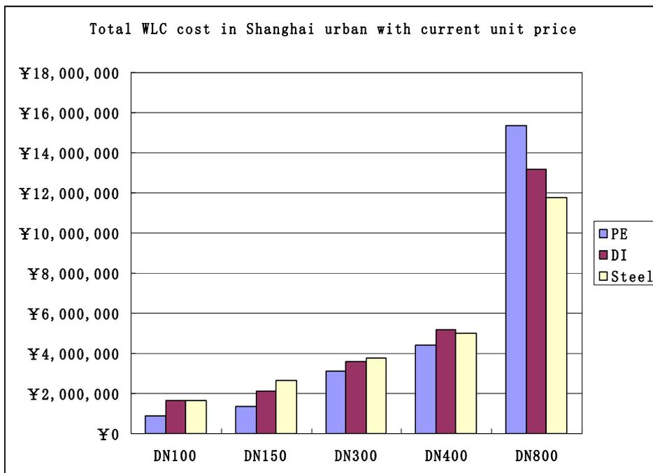
The charts show that in both urban and rural situations PE pipelines have a lower whole life cost on pipelines having nominal diameters of up to 400 mm, but are more expensive at the largest diameter on DN 800.
