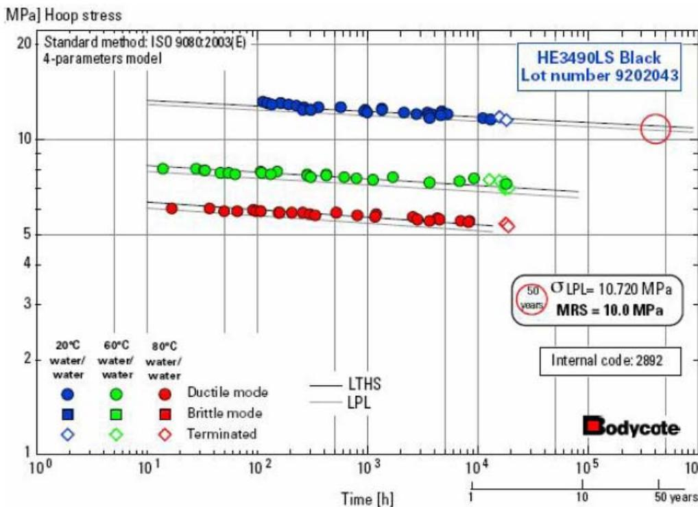
**Fig 6. A “tough” PE100 material that is suitable for gas and water pipe production**
