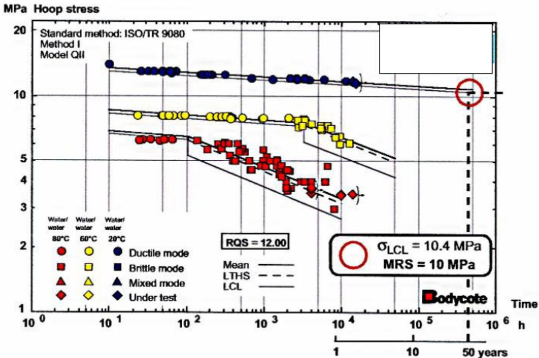
**Fig 5. A “brittle” PE100 material that is not suitable for gas and water pipe production**
