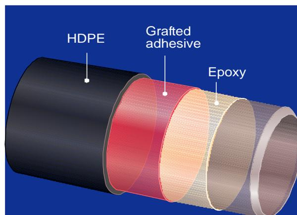
Fig 7. Typical 3LPE coating system
